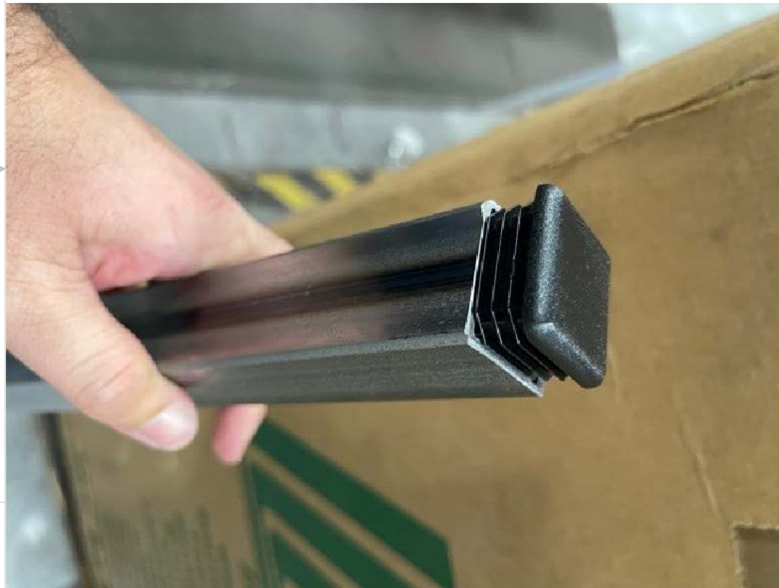
STEP 4: INSTALL CAP PLUGS TO BOTH SIDES OF EACH SEAT TUBE.
