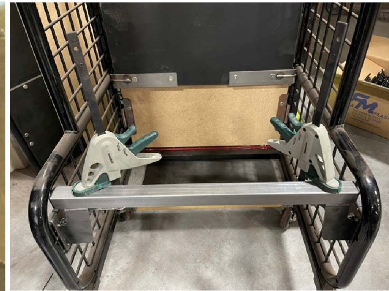
STEP 5: CLAMP TUBES TO BRACKETS AS SHOWN
