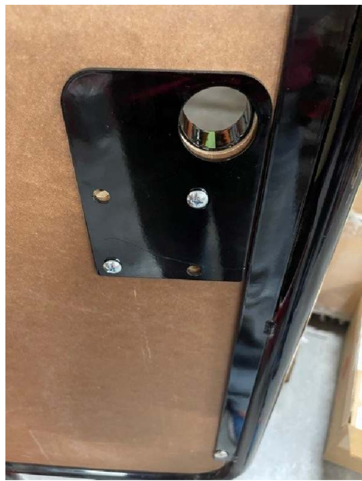
STEP 4 INSERT HANDLE WELDMENT TO FRONT FACE OF DOOR AND BACKER PLATE TO THE BACKSIDE OF DOOR. USE STANDARD NUTS ALONG WITH 1/4-20 X 3/4" PHILLIPS HEAD SCREWS TO SECURE.
