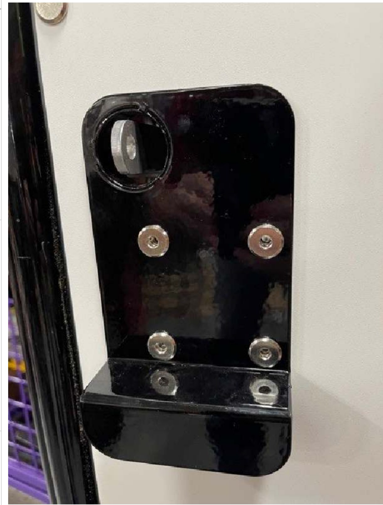
STEP 4 INSERT HANDLE WELDMENT TO FRONT FACE OF DOOR AND BACKER PLATE TO THE BACKSIDE OF DOOR. USE STANDARD NUTS ALONG WITH 1/4-20 X 3/4" PHILLIPS HEAD SCREWS TO SECURE.
